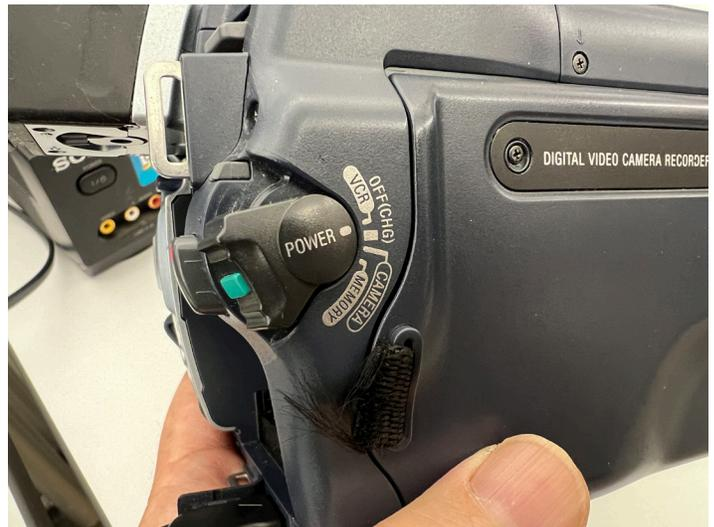
**Step 8:** Rotate the thumb wheel on the side of the camera to VCR by pressing the green button to release it.
