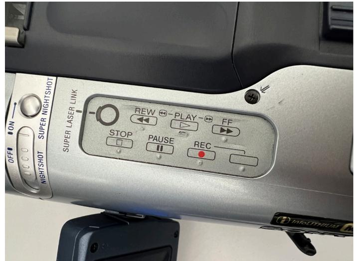
**Step 12:** Use the controls on the top of the camera to control the tape.
