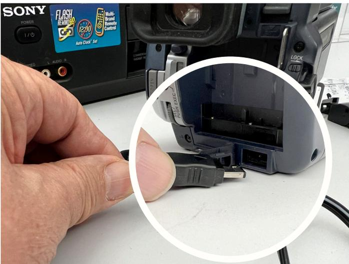
**Step 7:** Plug the other end of the power cable into the connection at the back of the camera.
