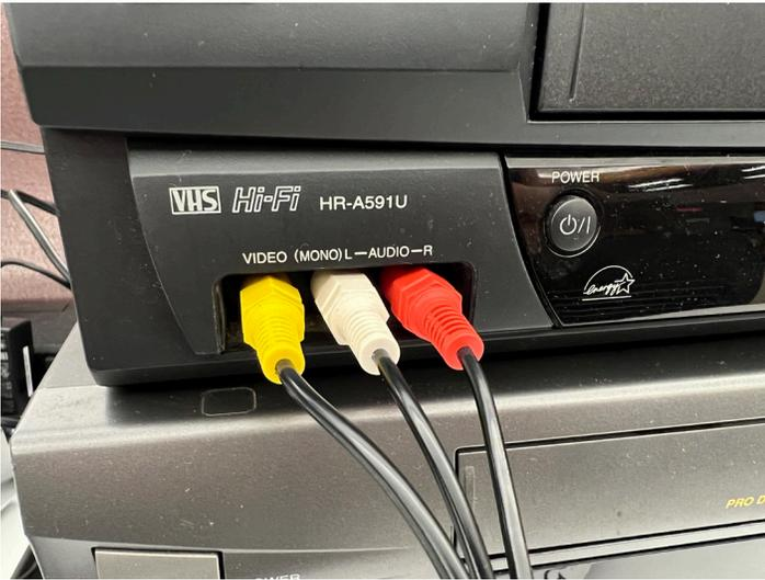
**Step 5:** Connect the other end into the front connection of the VCR that is connected to the computer.
