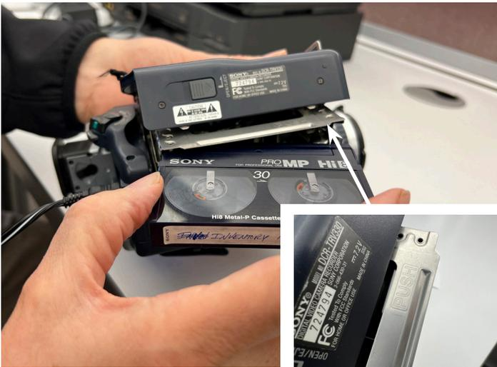
**Step 11:** Insert the video cassette and carefully push where indicated. The mechanism will automatically begin to close. Once closed, snap the black cover back in place.
