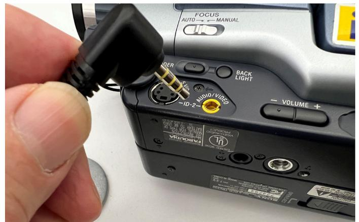
**Step 4:** Insert the mini plug into the yellow A/V connection.
